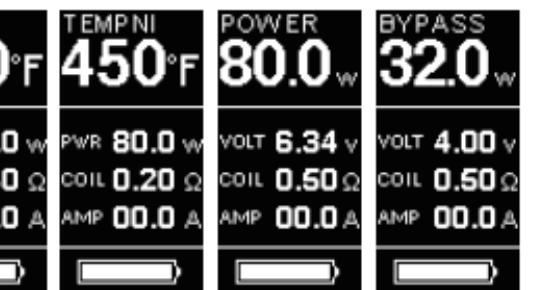
2. After pressing the fire button 3 times, the first row will flash to indicate you enter into the menu.
